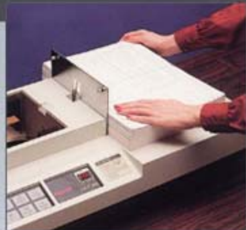
The LOOP PLUS automatically tensions, seals and cuts the strapping in just seconds.
