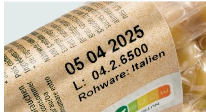
Variable data such as ingredients, price, barcode, or "best before" date is printed "on demand" in the space provided on the band during the banding process.
